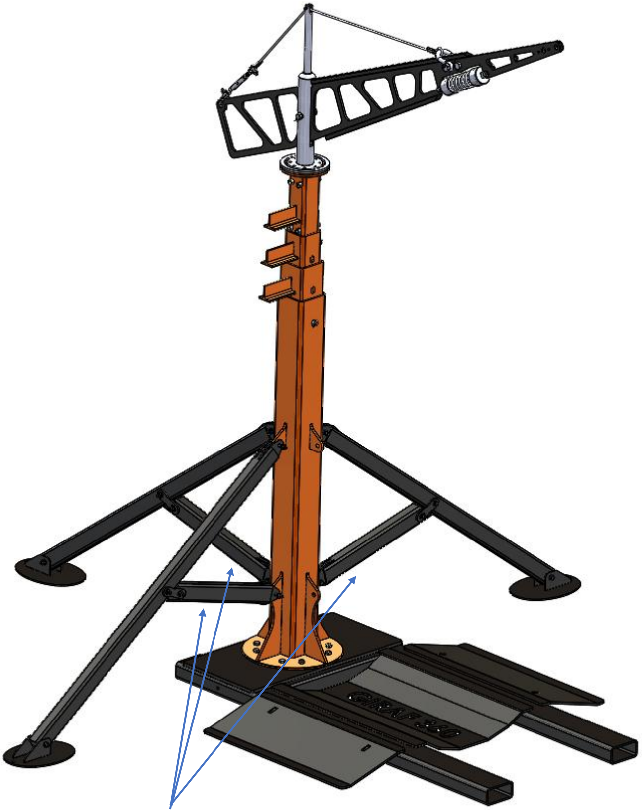
9. Short Support Profiles are connected between Long Support Profile and Tower 7000 part.
