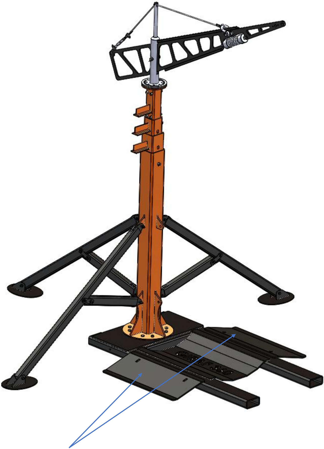
10. Ramps are placed after placing them on the ramp holders.
